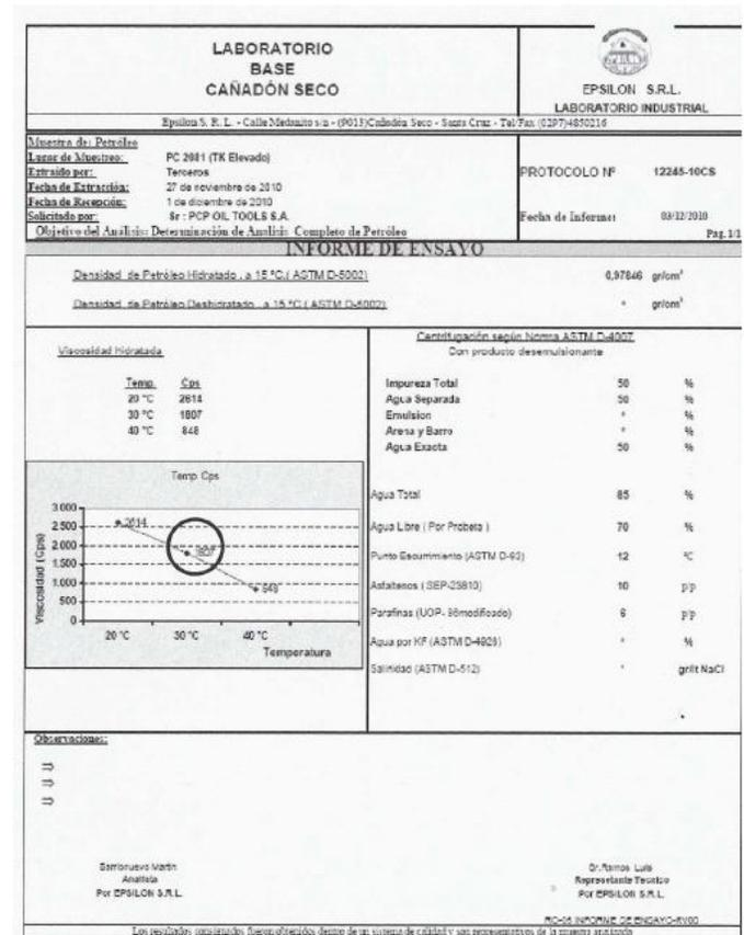
Figure 4. Laboratory measurement of viscosity at the well head after installation of the downhole passive energy technology tool. Well head viscosity was reduced from 7730 cps to 1807 cps following installation of the downhole tool.
