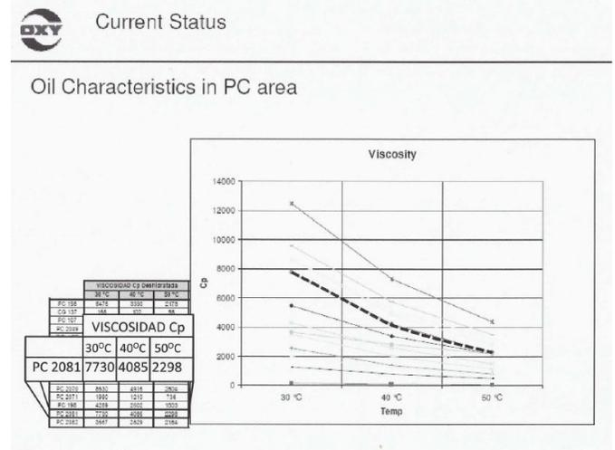
Figure 3. Viscosity measurement at the well head in PC 2081 before installation of the downhole passive energy technology tool.
